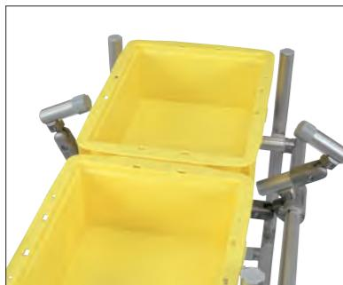
1 Back Stopper (both side) is in the open position when there is container intake on a Flip-Flop Table.
