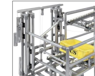
3 After Elevation table descends to the bottom and discharged container the weight will bring it back up.
