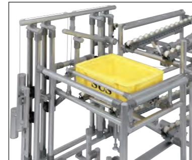
2 When the container intake, Roller that installed in between Green Frame L slot will help Elevation Table moves down smoothly in horizontal position.
