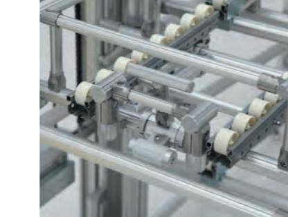
**3** When Elevation Table comes all the way down, Corocon part will slope to discharge container.
