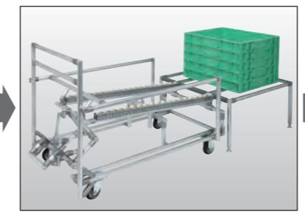
3 After move container on to a rack and return the pedal, Corocon part tilts back to the position waiting for a new feed container.
