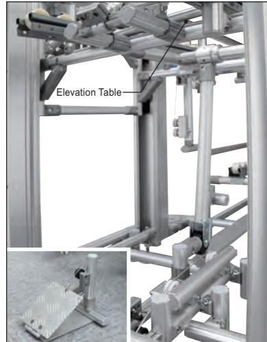
1 Frame of strut stopper will lock due to its function when there is container set on the table, and will stop Elevation Table coming down.
