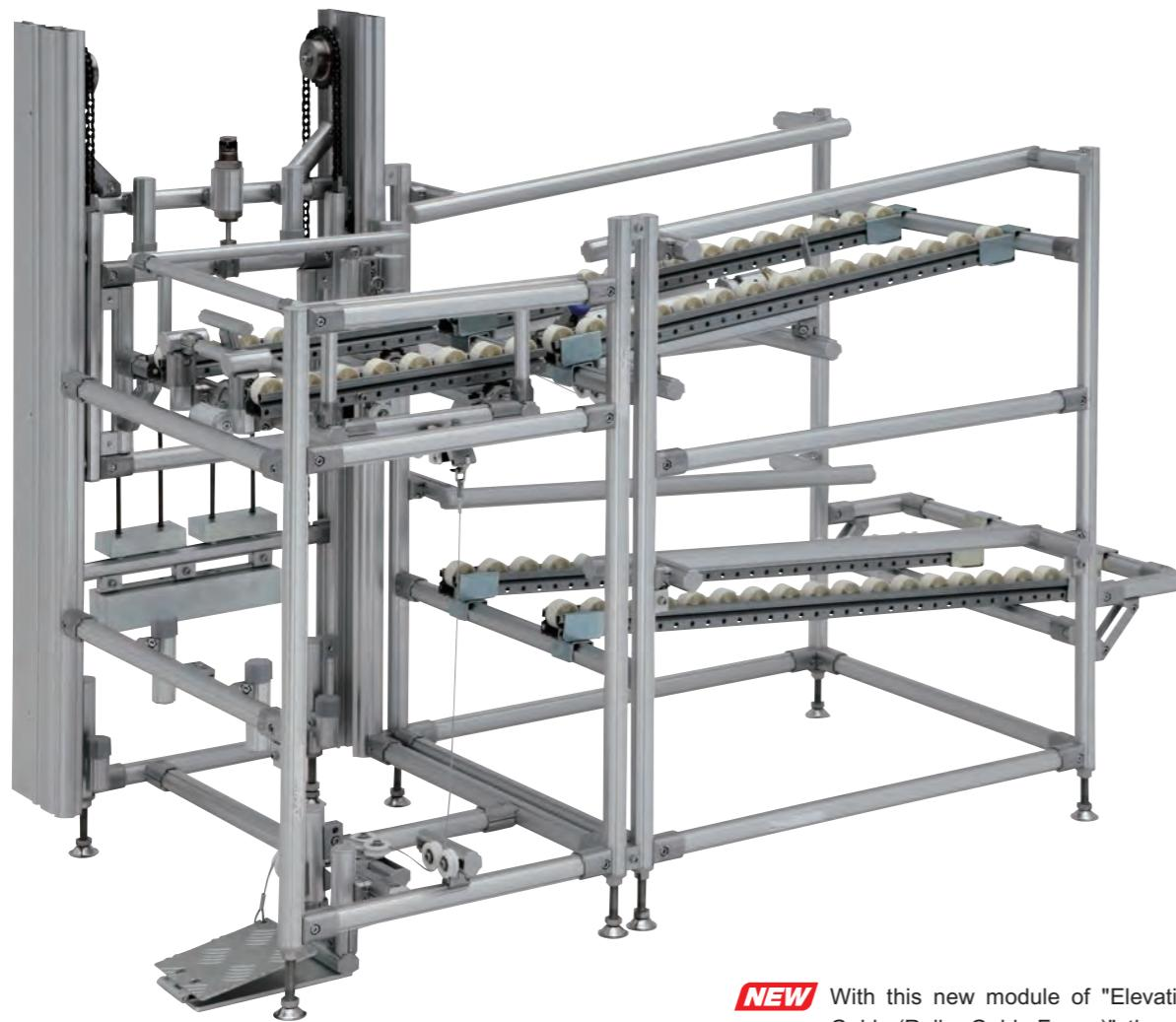
**NEW** With this new module of "Elevation Guide (Roller Guide Frame)", there is no longer need to adjust the elevation rail, which can be a smooth construction.
