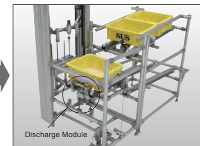
2 When the table come all the way down, the discharge module will eject the container to discharge.
