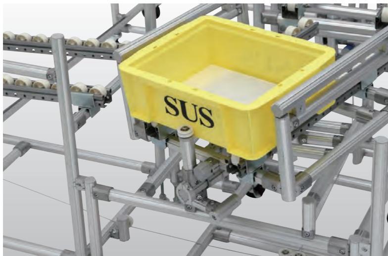
■ It is a stopper which has 90° Turn Module installed to control container holding and discharge.
