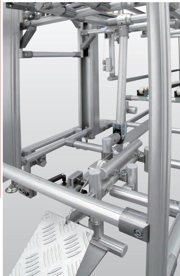
■ It is a system of lock and unlock Elevation Table at the top by kicking support frame with Foot Pedal.
