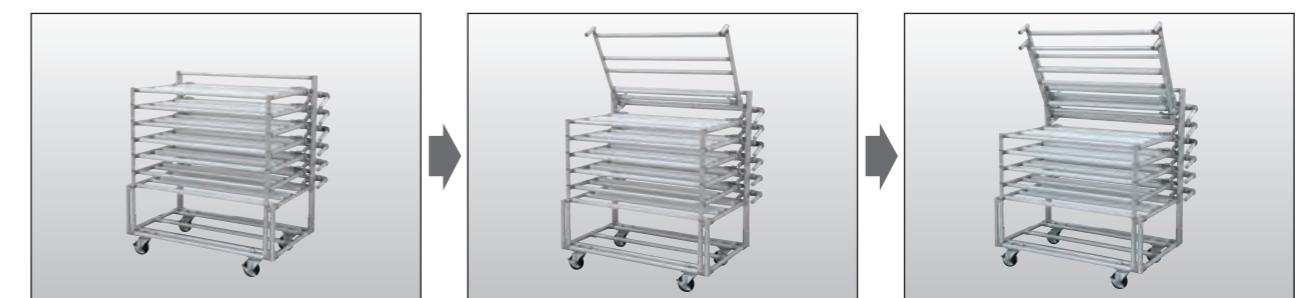
1 Remove all the work out from a rack to be empty, then flip it up over the head.
