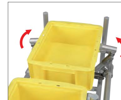
2 The Intermittent Stopper that linked to the movement of Flip-Flop Table, will rotate and the front stopper will unlock and discharge container. Additionally, the next container will be pushed by the back stopper.
