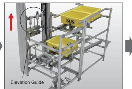
3 Table will elevate by the weight that was set at the Elevation Guide Module.
