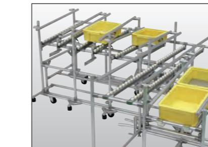
4 After Automatic Trolley moves forward, and AGV stopped at the container delivery position, Intermittent Stopper Module on Automatic Shooter side will be release to discharge container in to Automatic Trolley.
