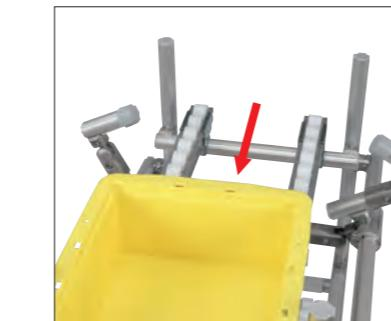
3 After container fully intake on a Flip-Flop Table, the back stopper (Both Side) will open again like in the step 1, and allow container to move forward.
