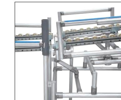
3 Stopper Module (Rotate) will fully unlock after table finished Rotate, then container will be discharged.
