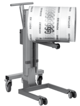
Compact lifter with V-block
