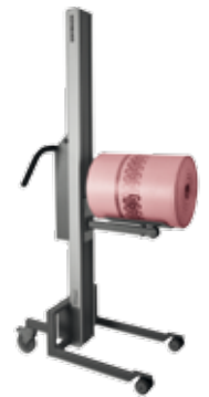
Lifter with combined boom and V-block
